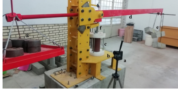
Figure 3: Components of apparatus and complete setup of new large consolidation device. a) camera, b) fix plate, c) Plexiglas cell, d) loading arm, e) loading weights, f) transfer load piston, g) balance weights.
