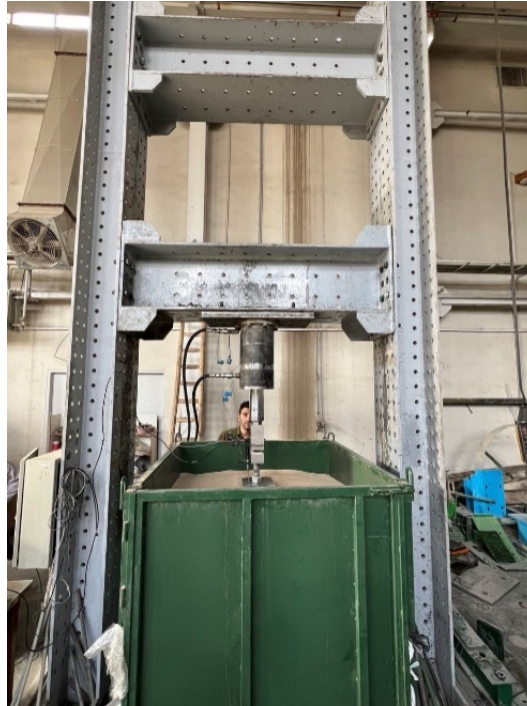
Figure 1: Experimental setup for the large-scale load testing of model micropiles embedded in a soil-filled chamber.
