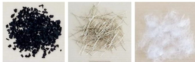
Figure 2: The appearance of polypropylene fibers, steel fibers, and tire-rubber particles
