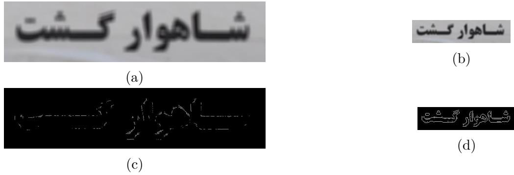
Figure 3: The effect of downscaling on edge map quality of blurred images, a) a blurred text image, b) downscaled version of a, c) edge map of the original image, d) edge map of the downscaled image
