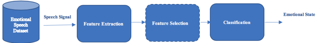
Figure 1: The basic block diagram of the speech emotion recognition system
