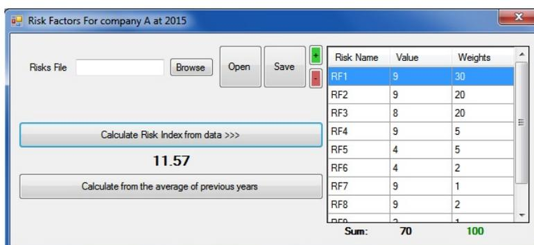
Figure 5: The data entry table of risk factors and calculation of risk index *RI*. in FGRM software
