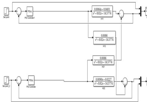
Figure 5: Simulink Model of Closed Loop Response of TTCIS
