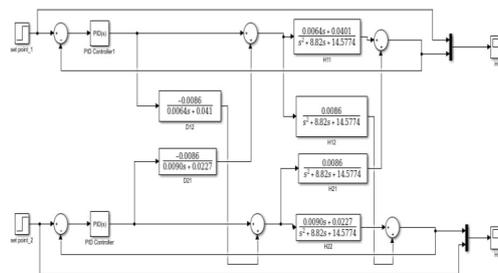
Figure 8: Simulink Model of closed loop response with decoupler
