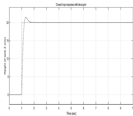
Figure 10: Closed loop response of tank 2 with decoupler
