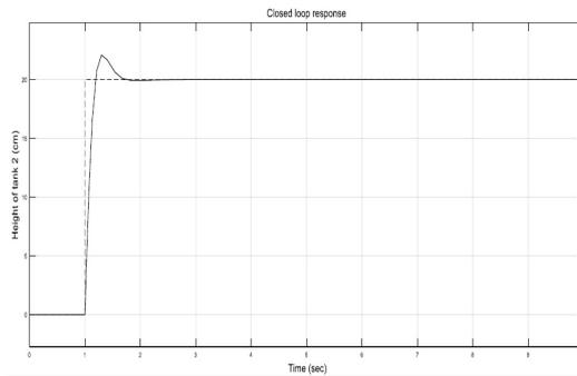
Figure 7: Closed loop response of tank 2 of TTCIS
