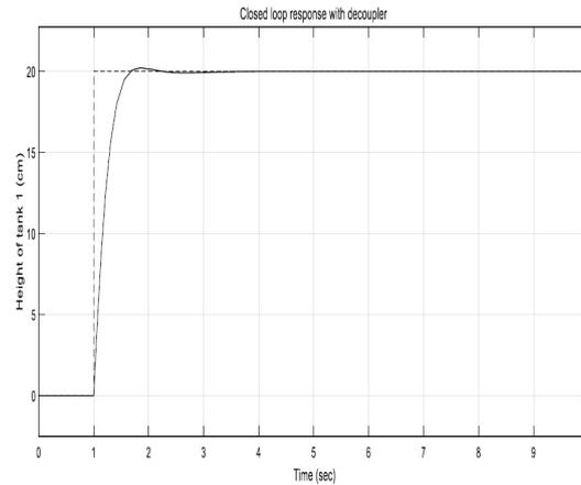
Figure 9: Tank 1's closed loop reaction with decoupler
