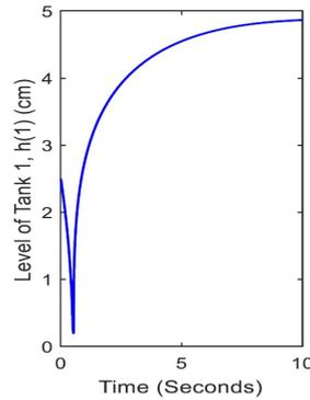
Figure 3: Open loop response of tank 1
