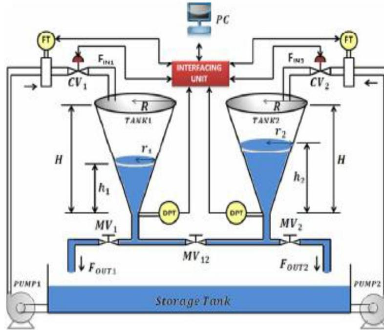
Figure 2: Schematic of TTCIS
