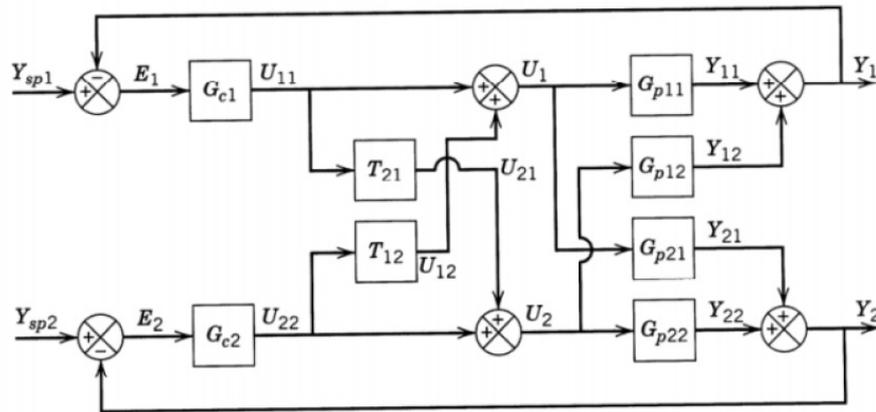
Figure 1: 2 × 2 Decoupling Control Scheme
