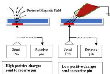
Figure 5: Process of collision detection sensor
