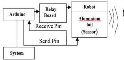
Figure 1: Block diagram of collision detection sensor
