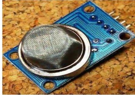
Figure 2: Alcohol Sensor
