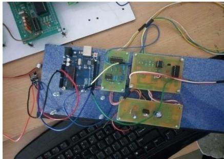
Figure 6: Smart helmet module
