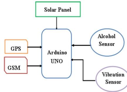
Figure 1: Block Diagram of Proposed Smart Helmet
