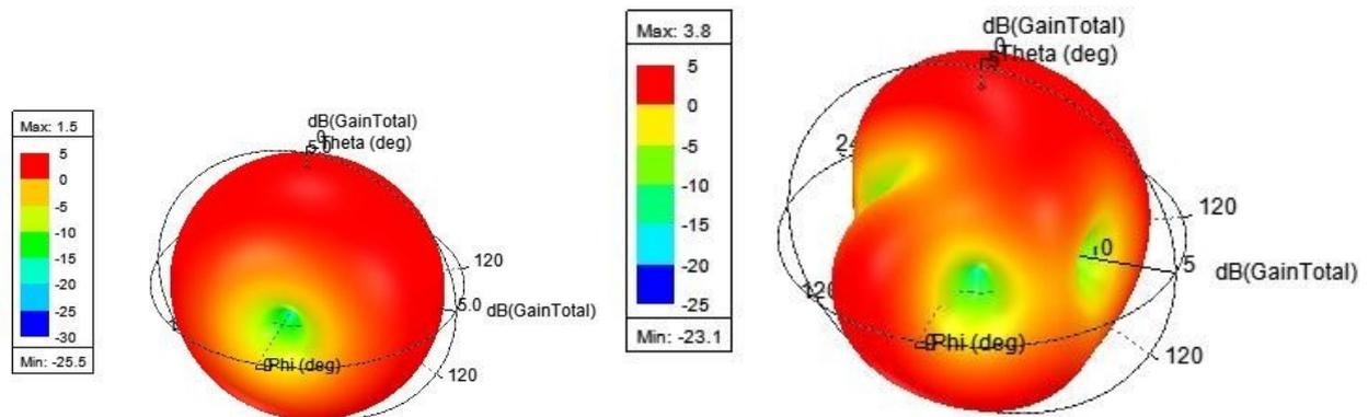
Figure 6: Gain at (a) 2.4GHz (b) 5.8GHz
