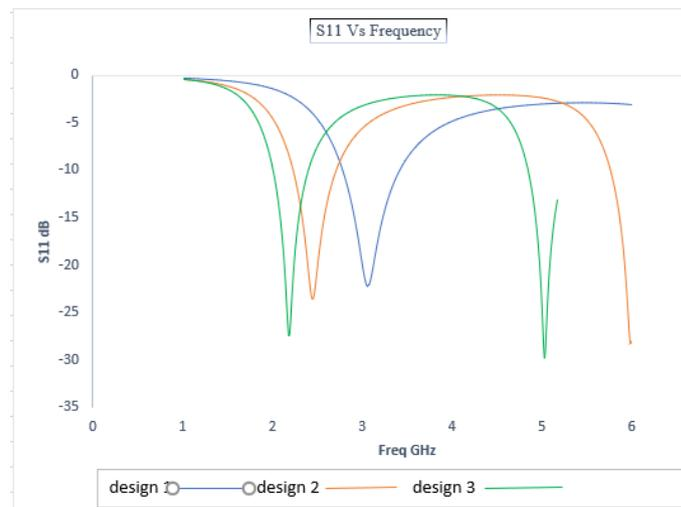
Figure 3:  $S_{11}$  of (a) design 1 (b) design 2 (c) design 3
