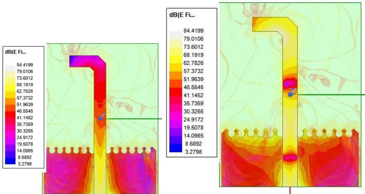
Figure 5: Surface current distribution (a) 2.4GHz (b) 5.8GHz
