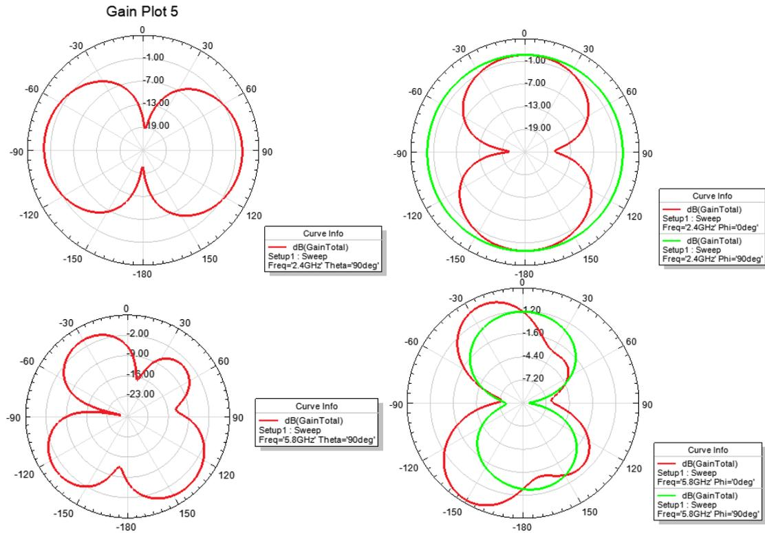
Figure 7: 8 Radiation pattern of Azimuthal and Elevation plane (a) 2.4GHz (b) 5.8GHz
