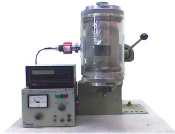
Figure 2: Thermal evaporation system.
