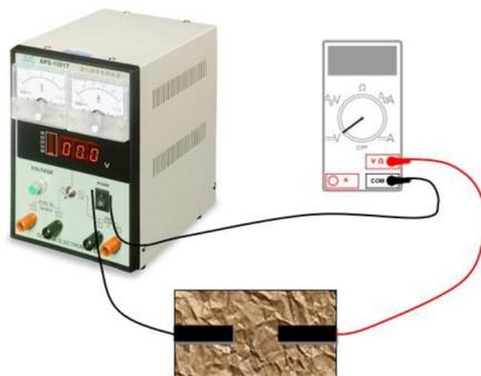
Figure 3: Electrical resistivity measurement system.
