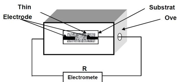
Figure 4: D.C. conductivity measurements system
