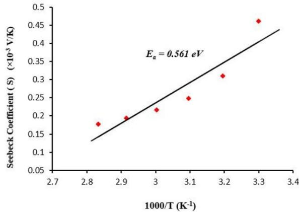
Figure 10: Temperature dependence of Seebeck coefficient for CdTe film
