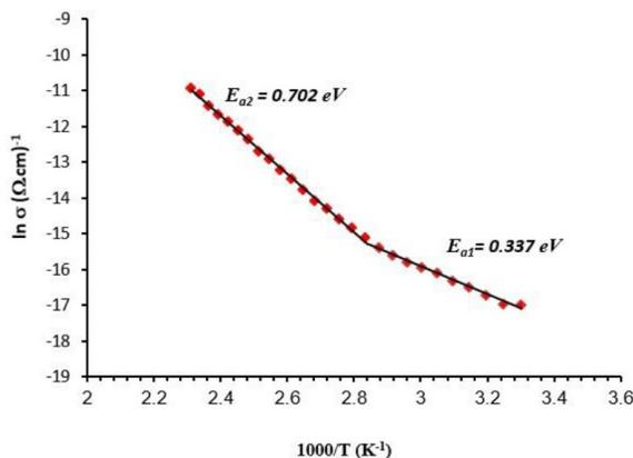
Figure 8: Variation of DC conductivity  $\ln \sigma$  with  $1000/T$  for CdTe films.
