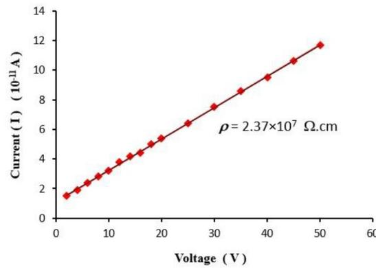
Figure 6: current – voltage plot of CdTe thin film
