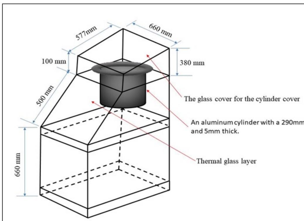
Figure 2: A simplified diagram of the steam sterilizer chamber.
