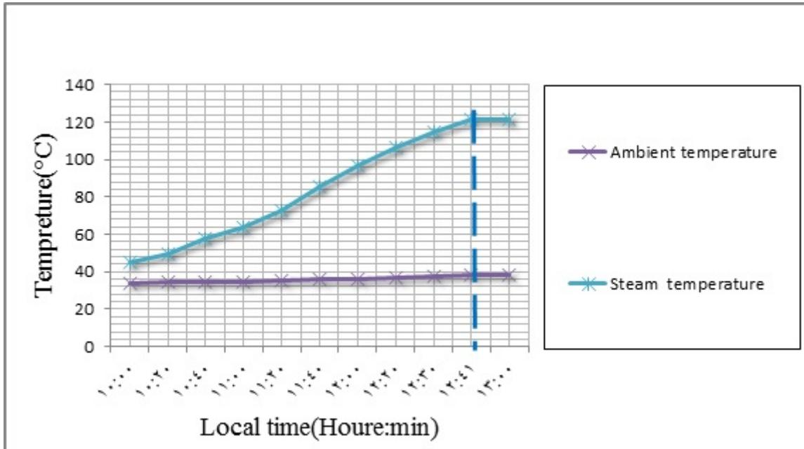
Figure 8: Steam temperature change inside cylinder over time with surgical instruments.
