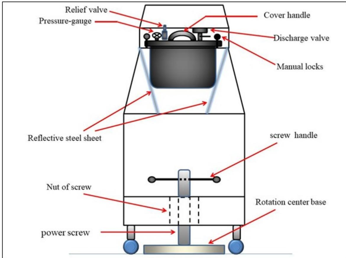
Figure 3: A simplified diagram showing front view of the final shape of the device.
