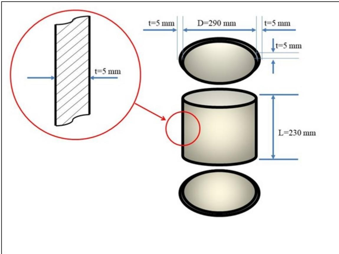
Figure 5: The dimensions of the steam sterilizer cylinder.
