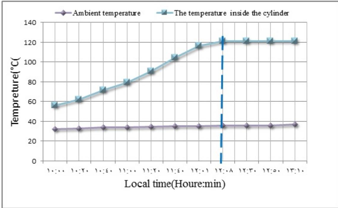
Figure 6: Steam temperature change inside the sterilization cylinder over time.
