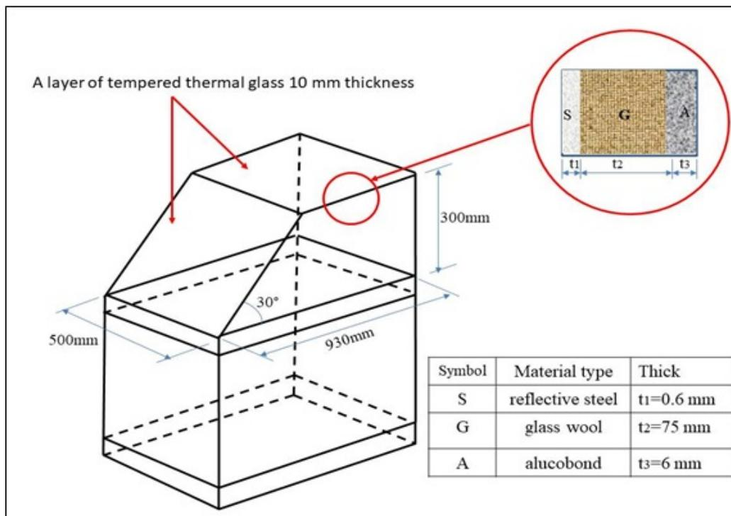
Figure 1: Schematic diagram of sterilization chamber details.
