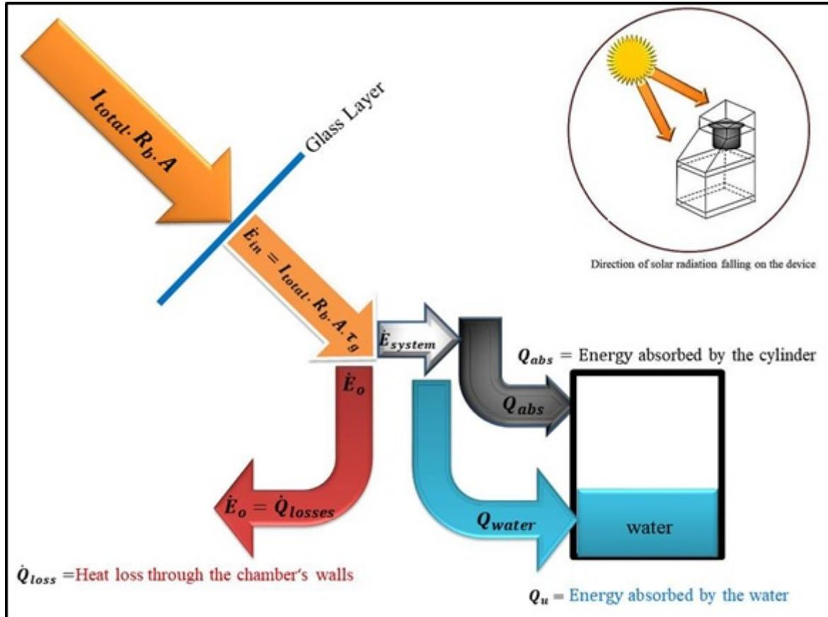
Figure 4: A simplified diagram of the Thermal Balance for the chamber.
