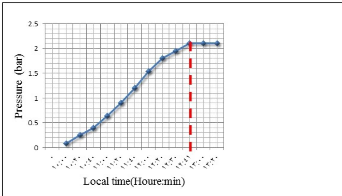
Figure 9: The pressure change inside cylinder over time with surgical instruments.
