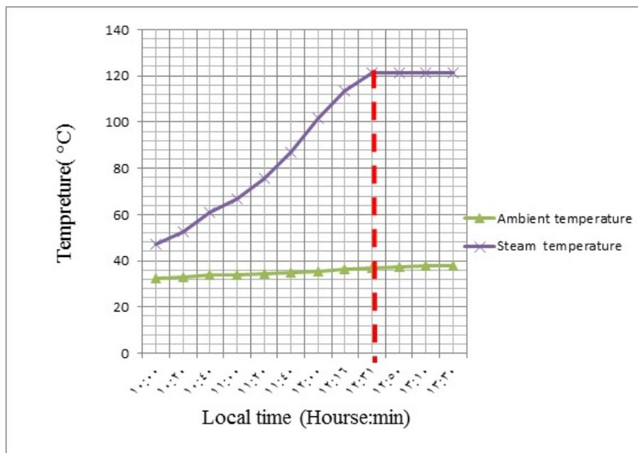
Figure 10: Steam temperature change over time with surgical instruments, and reflective cone.
