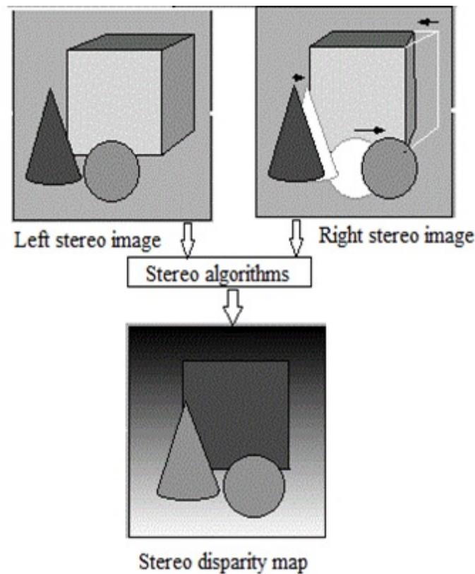
Figure 2: An example of stereo vision depth extraction
