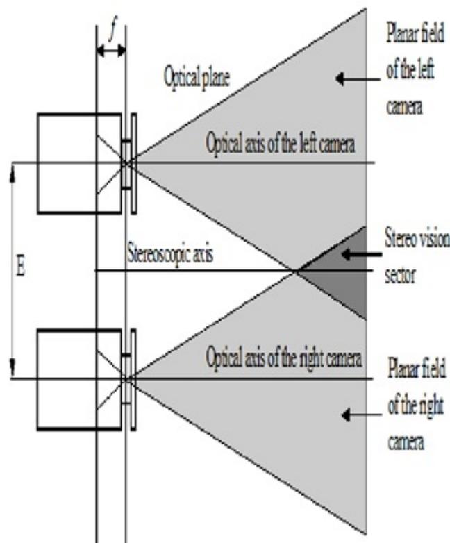
Figure 1: Stereo vision fundamental concept (Triangulation principle)
