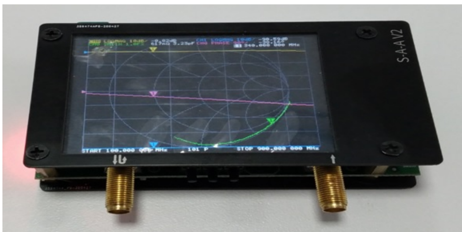
Figure 4: The Employed NanoVNA (S-A-A-V2) in this study
