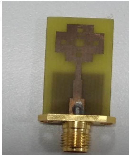
Figure 11: The reproduced prototype of the UWB antenna based on [12].
