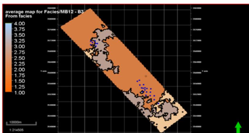
Figure A.13: Facies (Rock type) modelling for MB12 unit in Mishrif reservoir/ Buzurgan Oilfield.
