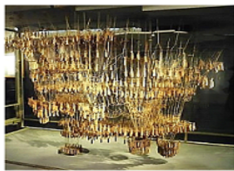
Figure (4). Antonio Gaudi, reproduced a model of "La Sagrada Família", 1983-1926. Upside-down structural analysis made from strings and weighted bags [11].
