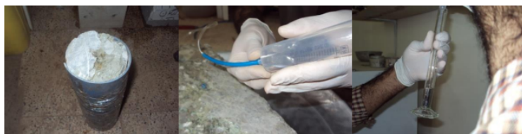
Figure 2: How to prepare and calculate the volume of the hole (cylindrical sample, measuring the volume of mercury, injecting mercury into the sample)
