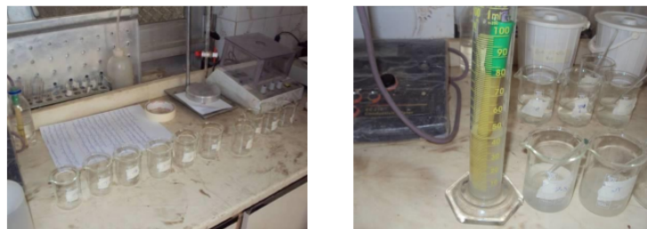
Figure 5: Experiment to determine the maximum amount of gypsum dissolved in Marash Dam water
