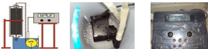
Figure 3: Tools and how to perform the circulation test for a cylindrical sample
