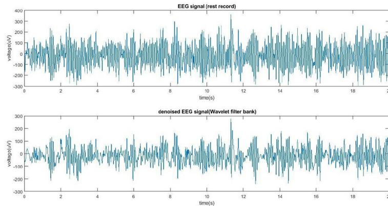
Figure 4: View of the used EEG signal before and after denoising optimized with SFO
