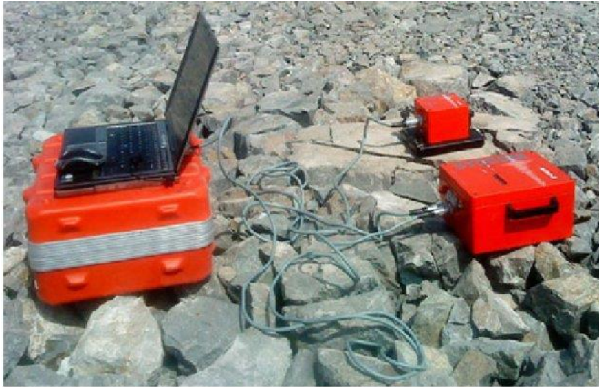
Figure 3: MR2002 geophone for ground vibration recording
