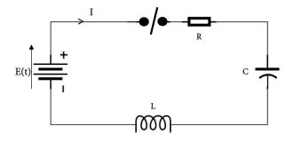
**Problem 3.4.** An inductance of 3 henry, a resistor of 16 ohms and a capacitor of 0.02 farad are linked in series with an emf of 300 volts. At t = 0, the charge on The circuit's capacitor and current are both 0. At any time, you can check the charge and current.t > 0.
