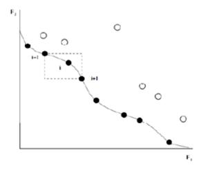
Figure 3: Calculation of a control parameter, i.e., crowding distance [7]
