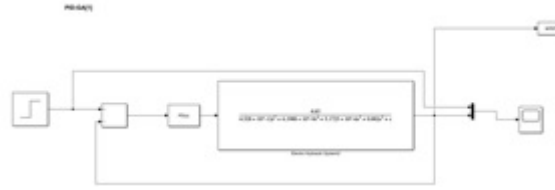
Figure 4: The overall block diagram of the electro-hydraulic position servo control system with GA optimized algorithm.
