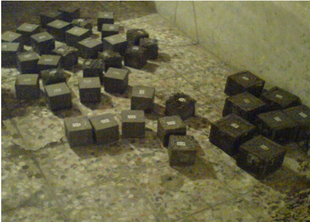
Figure 2: Preparation of specimens for ultrasound wave velocity monitoring test
