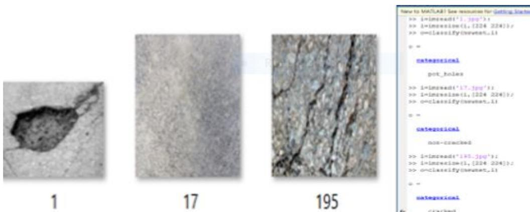
Figure 7: sample pavement images and the corresponding predicted output of the proposed model
