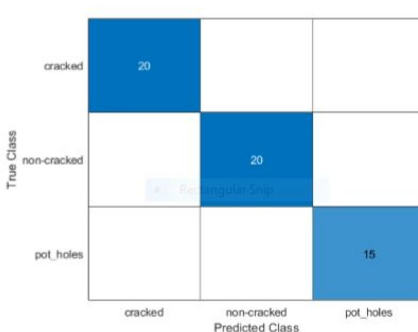
Figure 10: Confusion matrix chart for pavement crack detection system
