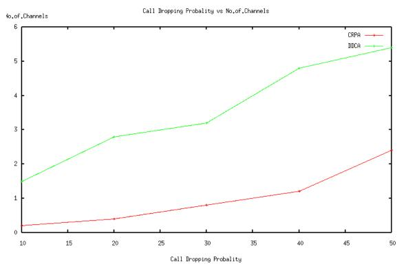
Figure 5: Call Dropping probability Vs No. of Channels
