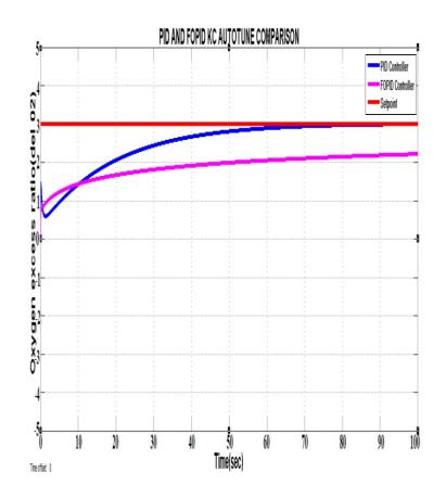
Figure 4: Comparison of PID and FOPID KC Auto tune of the system
