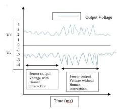
Figure 6: Sensor output waveform
