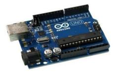
Figure 2: Arduino Board
