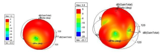
Figure 6: Gain at (a) 2.4GHz (b) 5.8GHz
