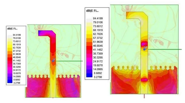
Figure 5: Surface current distribution (a) 2.4GHz (b) 5.8GHz
