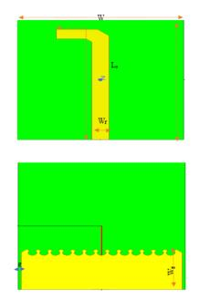
Figure 1: (a)Top view (b) bottom view of antenna
