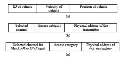
Figure 3: Frames Used (a) Beacon Frame (b) Request to Transmit Frame (c)Request to Hand-off Frame
