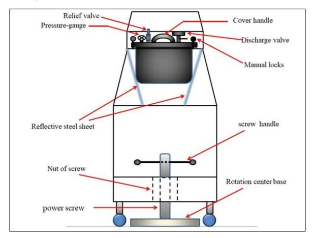
rotation, which is a rectangular base that was manually lowered by a screw to rest on the ground, as shown in Figure 3.
