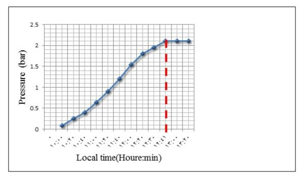
Figure 9: The pressure change inside cylinder over time with surgical instruments.
