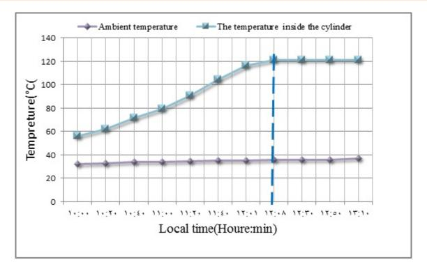
Figure 6: Steam temperature change inside the sterilization cylinder over time.
