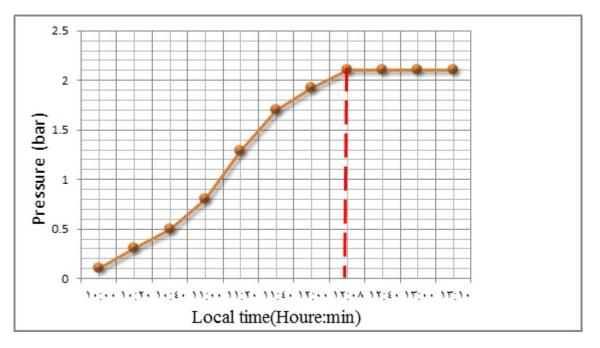
Figure 7: The pressure change inside the cylinder over time.
