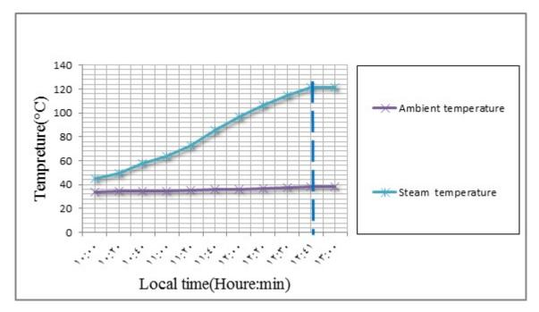
Figure 8: Steam temperature change inside cylinder over time with surgical instruments.
