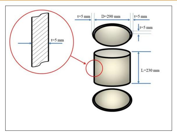
Figure 5: The dimensions of the steam sterilizer cylinder.
