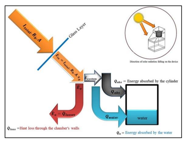
Figure 4: A simplified diagram of the Thermal Balance for the chamber.
