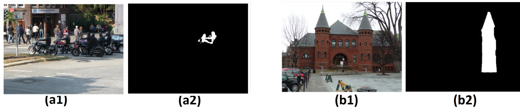
Figure 4: Example results of the BAM forgery detection algorithm on the IMD dataset. (a1) and (b1) Original image [13]. (a2) and (b2) Detected forged region
