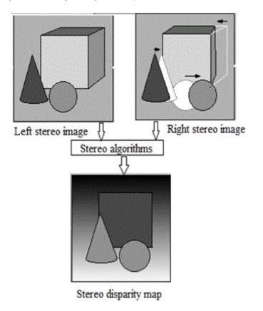
Figure 2: An example of stereo vision depth extraction
