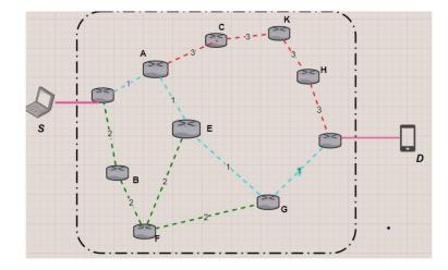
Figure 1: Schematic diagram of multi-path routing for MANETs
