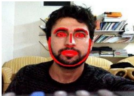
Figure 5: Key face characteristics in an image are labeled and identified using facial landmarks
