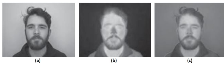
Figure 3: Three types of images were combined using the discrete wavelet transform (DWT): (a) visual, (b) thermal, and (c) sensor-level image [19].
