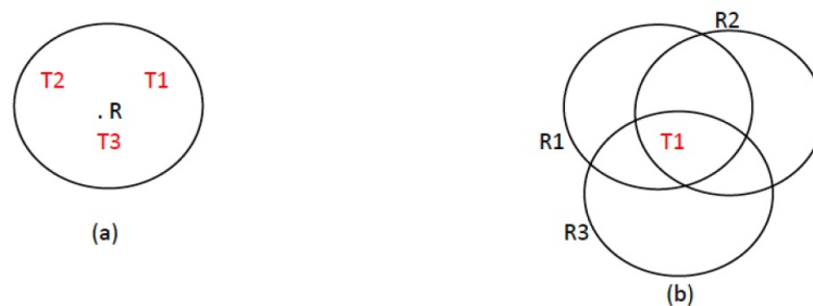
Figure 2: (a) Tag collision problem. (b) Reader collision problem
