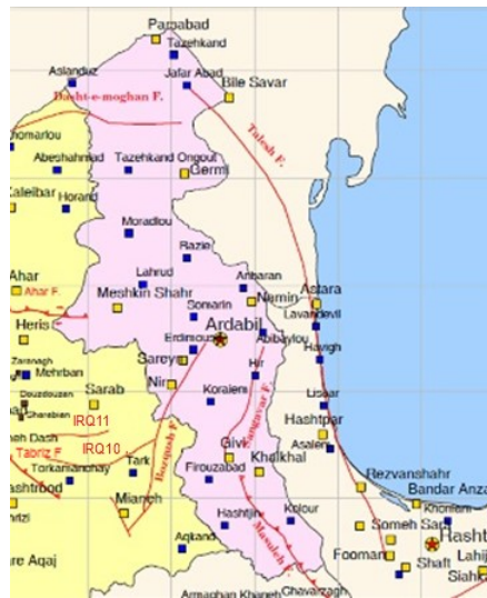
Figure 7: Active fault zones in the Ardabil Province and its vicinity (Water and Wastewater Company)
