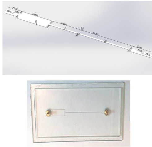
Figure 2: Dimensions of manufactured microchannel in terms of mm (the perpendicular dimension of the plane is 200 \mu\text{m} ) and Manufactured microchannel (top view).
